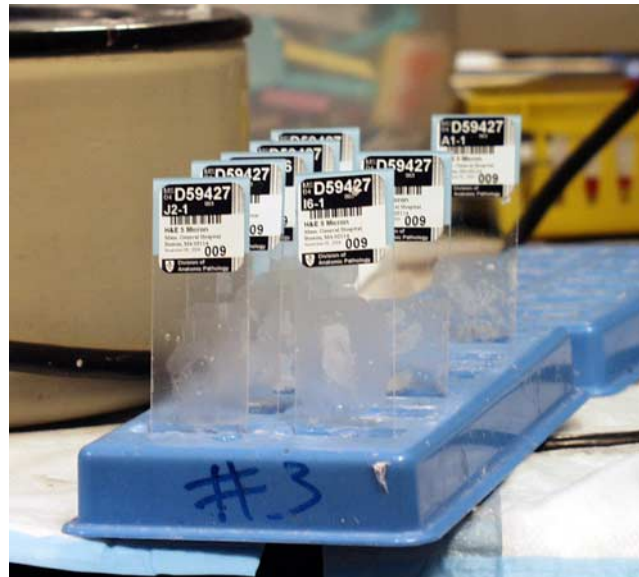
Slides await to be processed in the stainer. Each slide is individually identified with specimen-specific data and barcodes printed on a StainerShield label at the cutting station.
